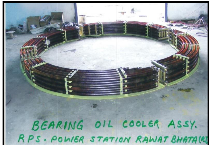
HYDRO GENRATOR BEARING OIL COOLER
